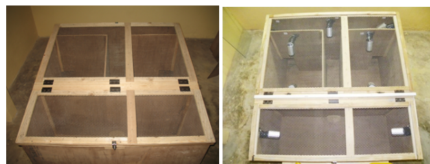
Figure 5: Snake repellent evaluation chamber (before and after fitting CCD cameras) as viewed from above
