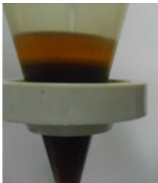
Figure 12: Upper layer shows biodiesel and lower shows glycerin.
