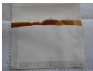
Figure 11: Paper chromatographic technique of different oil sample.
