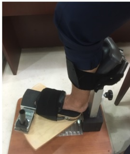
Figure 1B: Image of the syndhoo device from the side with the foot placed on the rotating board in neutral position.
