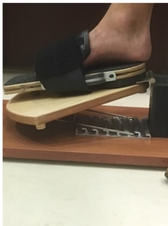
Figure 1C: Image of the syndhoo device from the side with the foot placed on the rotating board in 20 degrees of plantar flexion.
