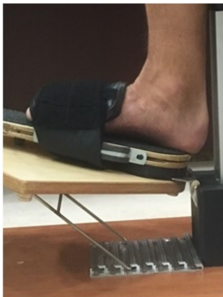
Figure 1D: Image of the syndhoo device from the side with the foot placed on the rotating board in 20 degrees of dorsiflexion.
