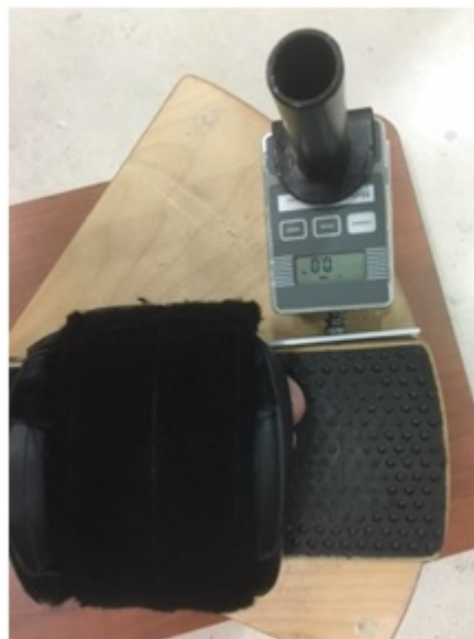
Figure 1F: Overview image of the dynamometer, linked to the rotating board.
