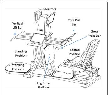
**Figure 1:** Bio Density<sup>™</sup> equipment (line art and photo) and the four exercise positions: 1) chest press (CP); 2) leg press (LP); 3) core pull (Core); and 4) vertical lift (VL).
