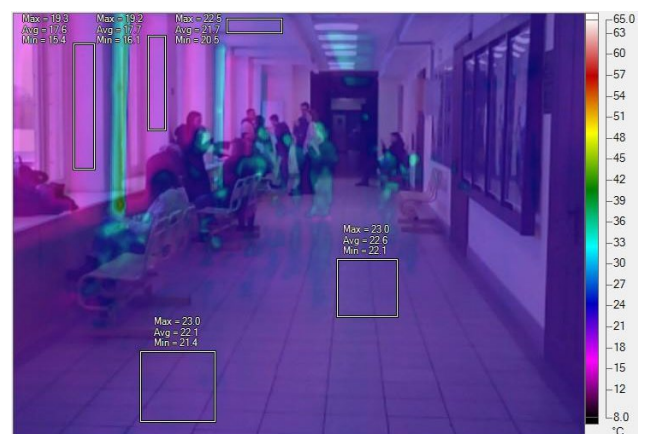
Figure 9: Group (b) radiators surrounding effect on the walls and the floor; (Amaish, Personal collection, Dec 2022).
