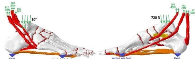
Figure 3: Boundary and loading settings applied to the foot model
