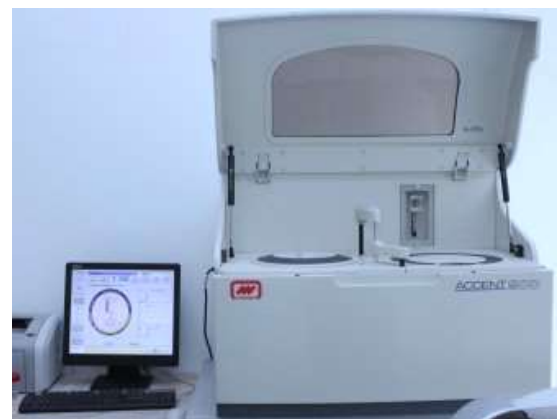
Fig.1. Automatic Biochemistry Analyzer / For Clinical Diagnostic / Benchtop Accent-2000.
