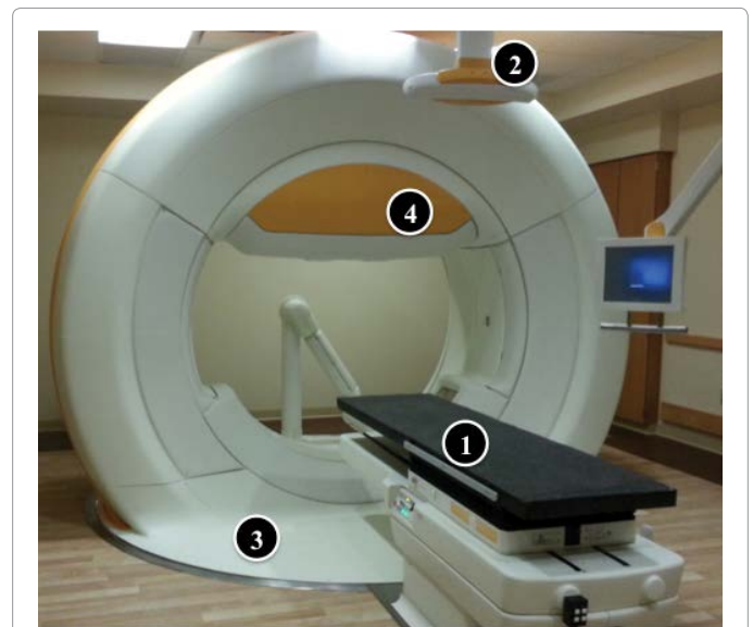
Figure 1: Vero SBRT. (1) Robotic tabletop. (2) Infrared camera. (3) Robotic O-ring gantry. (4) Gimballed accelerator.
