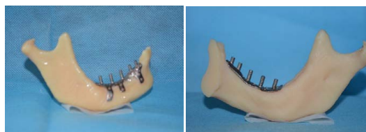
Figure 8: 3D printed mandible of the patient to check adaptation of the implant.
