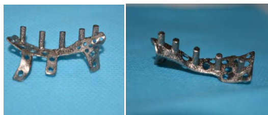
Figure 7: 3D printed subperiosteal implant with titanium.
