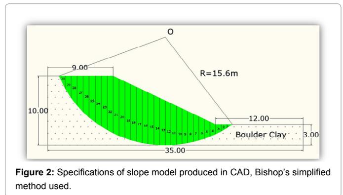
Figure 2: Specifications of slope model produced in CAD, Bishop's simplified method used.
