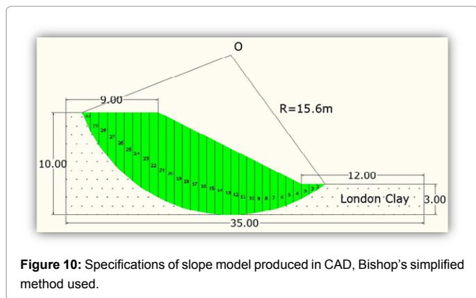
Figure 10: Specifications of slope model produced in CAD, Bishop's simplified method used.
