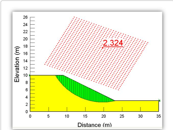
Figure 5: Slope model produced by SLOPE/W, indicating the minimum Factor of Safety.
