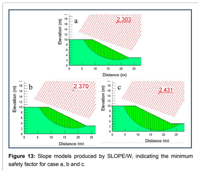
Figure 13: Slope models produced by SLOPE/W, indicating the minimum safety factor for case a, b and c.
