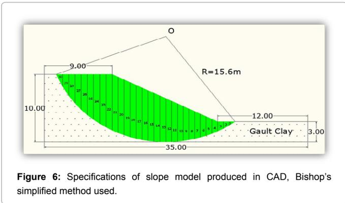
Figure 6: Specifications of slope model produced in CAD, Bishop's simplified method used.
