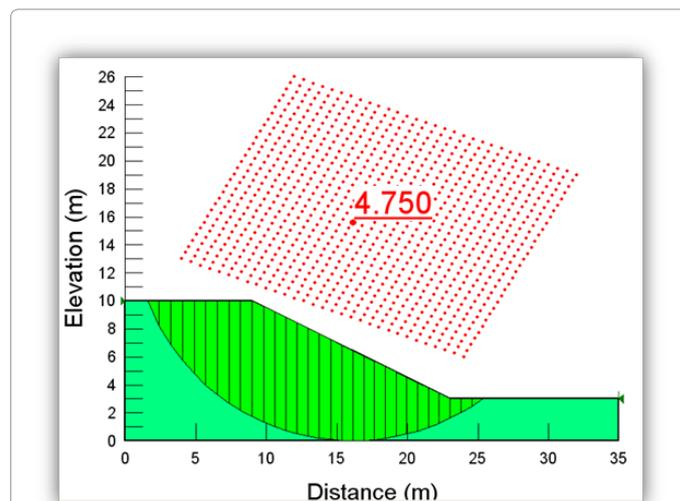
Figure 11: Slope model produced by SLOPE/W, indicating the minimum Factor of Safety.
