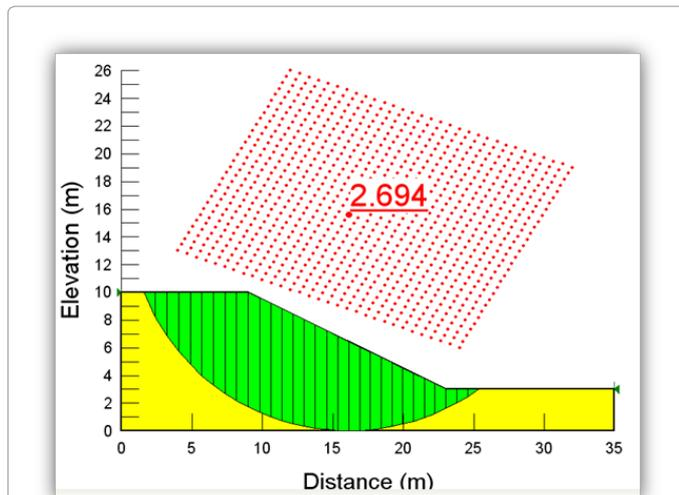
Figure 3: Slope model produced by SLOPE/W, indicating the minimum Factor of Safety.
