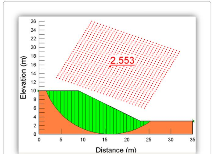
Figure 7: Slope model produced by SLOPE/W, indicating the minimum safety factor.
