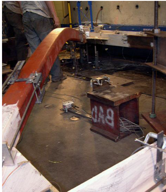
Figure 16: Brace buckling deformation.
