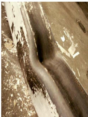
Figure 20: Initiation/Progression of tearing.
