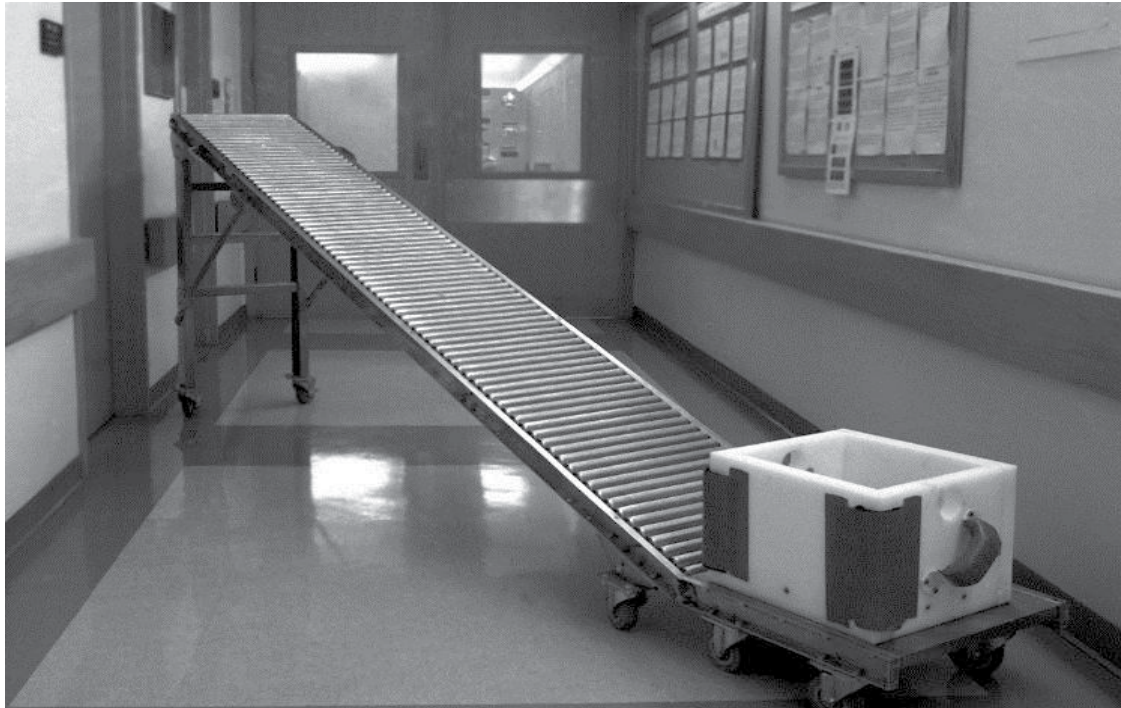
Figure 1: Repetitive lifting exercise ergometer consisting of a roller apparatus of the type normally used for moving boxes in a warehouse (3.3 meters in length, 1.32 meters high at upper end and 0.13 meters at lower end). The box (12 inches × 12 inches × 16 inches) was constructed of high molecular weight plastic (1.5 inches thickness) with handles mounted at 45° angles. The box weight (45 pounds) was augmented by mounting circular weights (20 pounds) with a threaded nylon rod.
