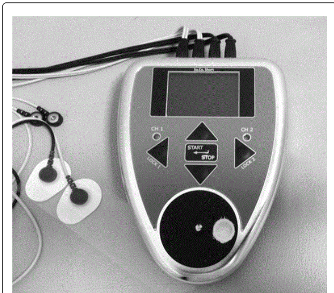
Figure 2: So.co.Short device. This interface allows the patient the following controls: total duration of the session; variations in the activity of channels 1 and 2; adjustment of the pulse voltage; duration of the therapy phases with information on the active signal emission times for the physiological response.
