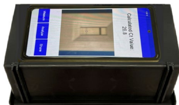
Figure 2: Photograph of a smartphone on cassette holder used to measure the Ct values on the test line of the LFA cassettes.
