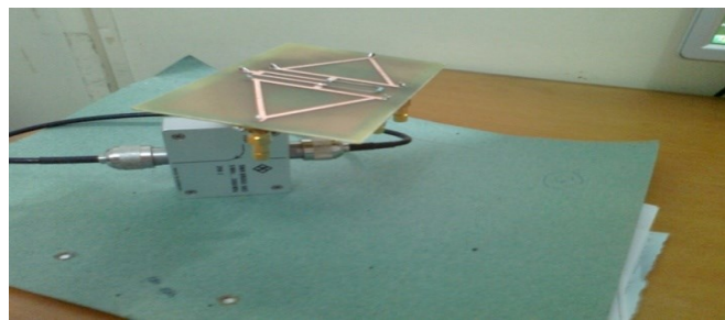
Figure 11: Measurement setup for the calculation of return loss at port 1.
