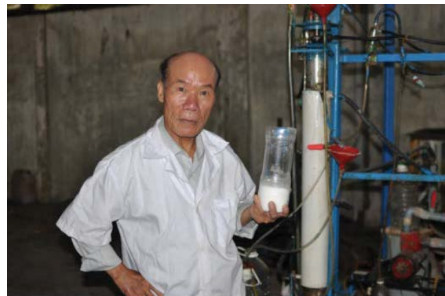
Figure 3: Nguyen [11] next to the experimental scheme to study the reaction between CO 2 and soda solution when using the new reactor operation continuously. In the hands of the professor is the crystal NaHCO 3 is the product obtained.
