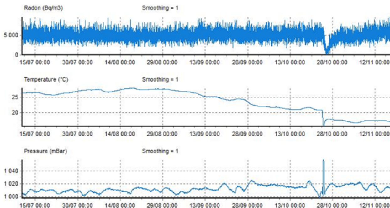
Figure 2: The signals recorded by the telemetric station of Figure 1. From the top: evolution of (a) radon (b) temperature and (c) air pressure. The output was produced by the software provided by the manufacturer.
