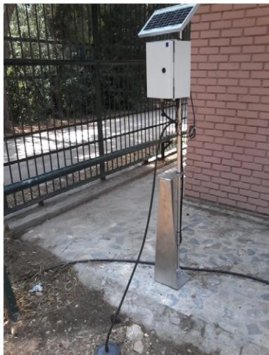
Figure 1: Radon telemetric station. The station comprises a solar panel, an IEEE box that contains all electronic equipment and the telemetric 3G emitting instrumentation. The BCM2 probe is enclosed in a closed PVC container and is immersed 1m below the ground.
