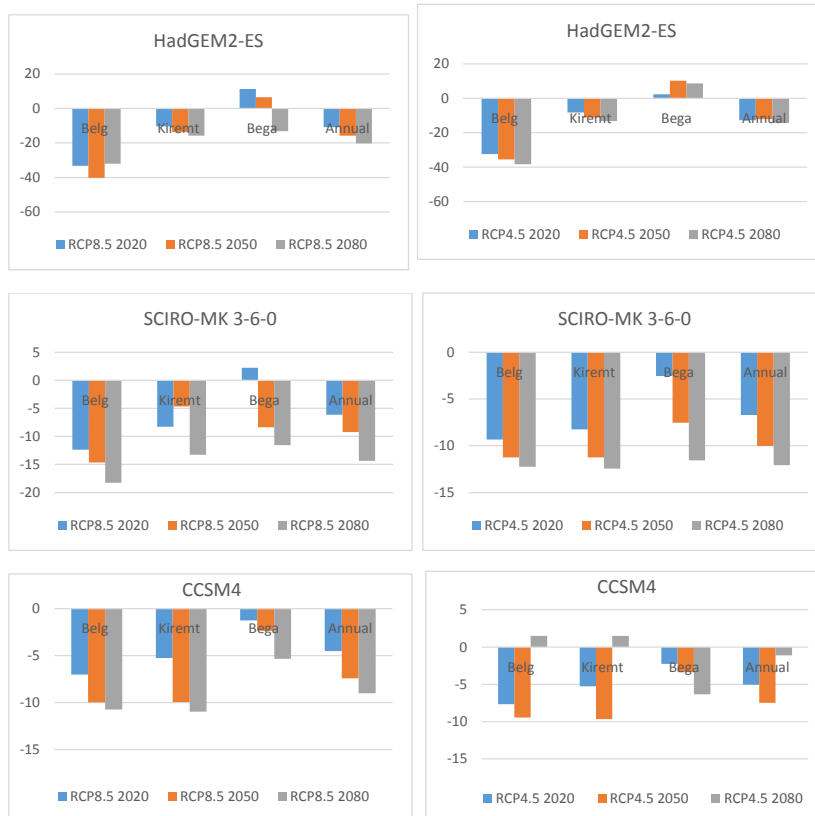
Figure 13: Percentage change in seasonal and annual inflow at Meki River with respect to baseline period for the HadGEM2-ES, CSIRO-MK 3-6-0 and CCSM4 model.
