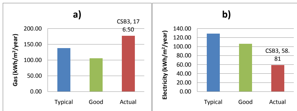
Figure 17: CSB3 (a) Gas consumption and (b) Electricity consumption vs. benchmarks.
