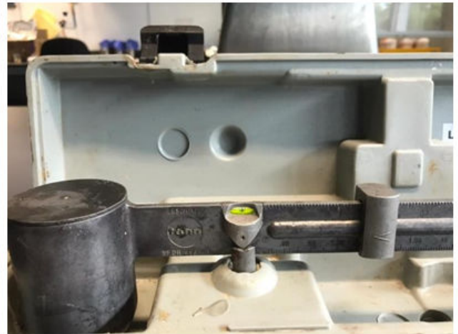
Figure 13: Reading taken when bubble in the level glass is in the middle.
