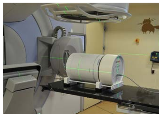
Figure 2: Phantom ArcCHECK and measurements facility.
