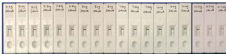
Figure 2: Photograph of LFAs used to measure 0 to 10 ng/mL tacrolimus spiked in saliva (12.5 and 25 ng/mL cassettes not shown).
