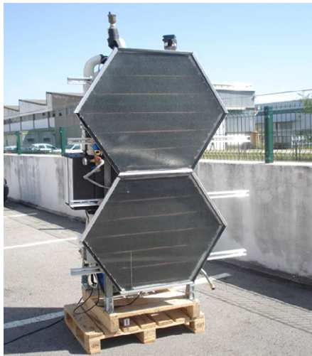
Figure 16: Thermodynamic heating water supply prototype.
