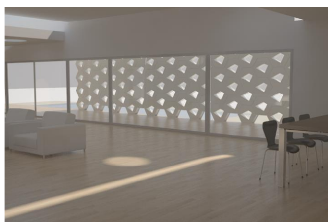
Figure 15: Internal view of a facade composed with modular parts for inside illumination.
