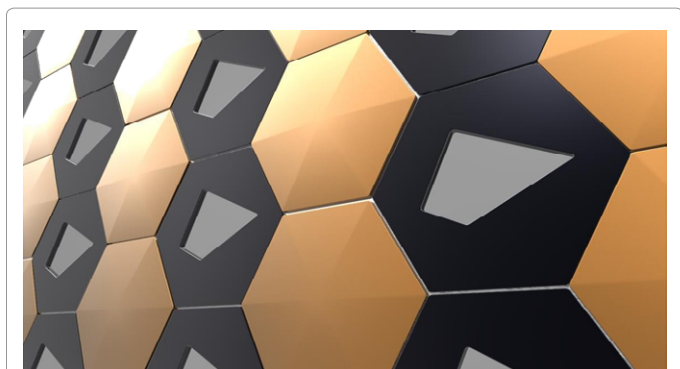
Figure 12: Simulation of a thermo-active surface built of copper and ceramic plus glass modules.
