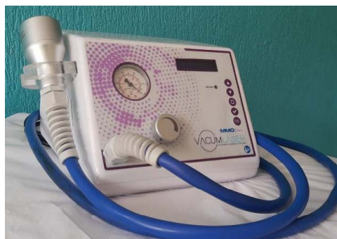
Figure 1: Vacuum-LASER, device that allows the simultaneous use of negative pressure and laser therapy on the same spot of application.
