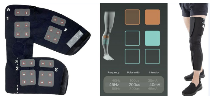
Figure 2: Cionic Neural Sleeve System. Left: Cionic Neural Sleeve showing the configuration of the FES and EMG electrode arrays; Center: Cionic mobile application interface for setting FES parameters (frequency, pulsewidth, intensity) and current field steering; Right: Cionic Neural Sleeve on body.
