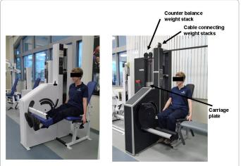
Figure 1: (a): The traditional concentrically based resistance exercise machine with a resistive weight stack that applies the same resistance during both phases of muscle contraction.
