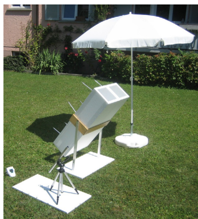
Figure 3: Twin-tubes from styrofoam.
