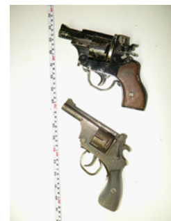
Figure 8: Country made revolver of .38" calibre.
