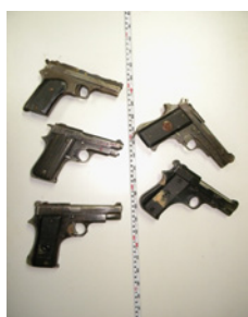
Figure 5: Improvised pistols of 7.65mm calibre.
