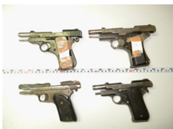
Figure 6: Improvised pistols with barrel lock condition.
