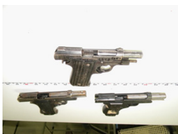
Figure 7: Improvised pistols with barrel lock above side.
