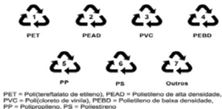
Figure 1: Symbology used to identify polymer packages. Standard NBR 13.230 of ABNT (Brazilian Association of Technical Standards)
