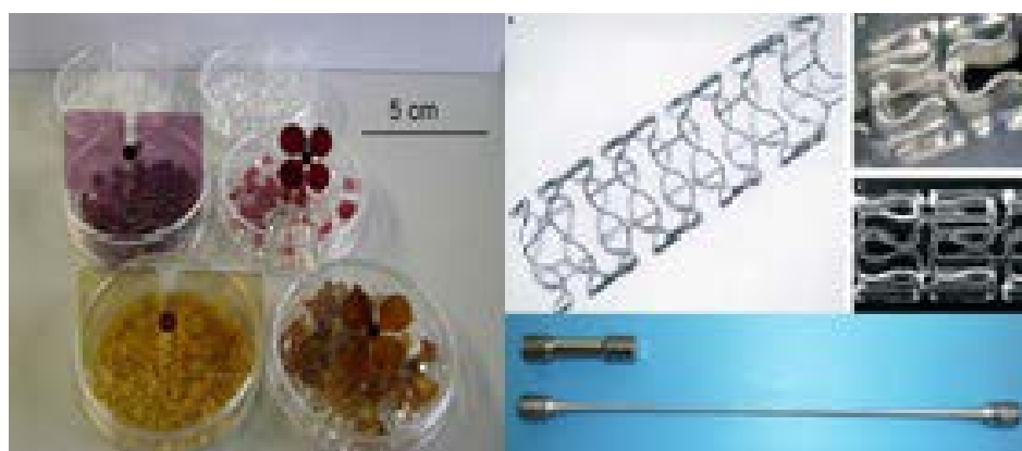
Figure 1: Laser-generated bioactive polymeric nanocomposites with embedded gold and silver nanoparticles on TPU-basis (left) titanium alloy and biodegradable magnesium with high tensile-strength and ductility (right).
