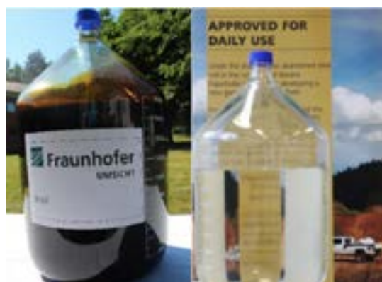
Figure1: Crude TCR ® -oil (left) and hydrotreated TCR ® -oil (right)
