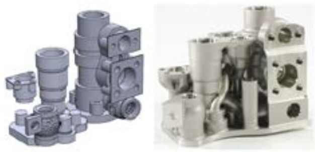
Figure 2: Positioned sub-components (left) and manufactured AM device (right).
