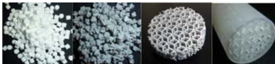
Figure 1: Examples of reactor packings: a) industrially used random packed bed elements; b) printed alternative with more complex shape; c) printed structured packing element; d) printed reactor tube with integrated structured packing.
