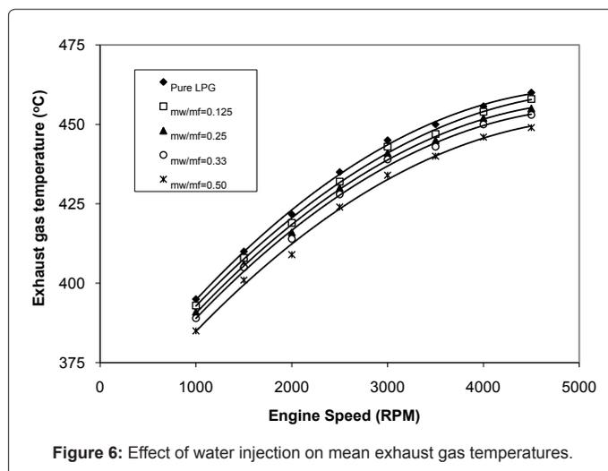
Figure 6: Effect of water injection on mean exhaust gas temperatures.
