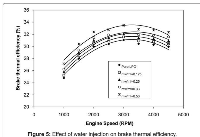
Figure 5: Effect of water injection on brake thermal efficiency.
